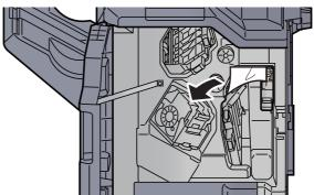
Q Return the conveyor guide (D1) to the original position.
