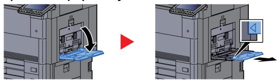
When loading paper sizes 12×18" and from A3 to B4 and Ledger to Legal, extend the support tray section of the multipurpose tray until the "\D" mark is fully appeared.
