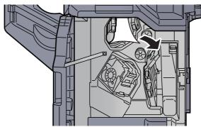
Q Return the conveyor guide (D4) to the original position.
