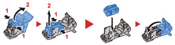
Install the Staple Cartridge Holder (B) or (C).
