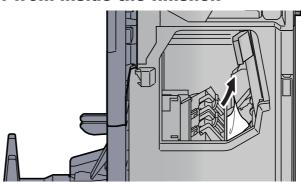
Remove the Staple Cartridge Holder (B) or (C).
