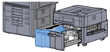
Pull out side feeder paper feed unit (B1).
