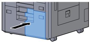
For Cassette 3 and 4, insert a sheet of the required paper size and type, as shown in the illustration.
