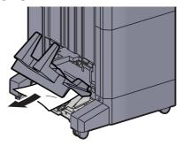
O Press the release lever to pull the folding unit out.
