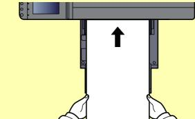
• After printing starts, catch the paper when it is output so that it does not fall.
