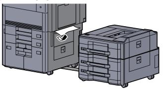
Open the side feeder top cover and the side feeder right cover 1.
