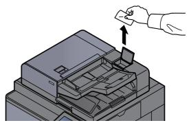
Clean the slit glass surface and the reading guide.
