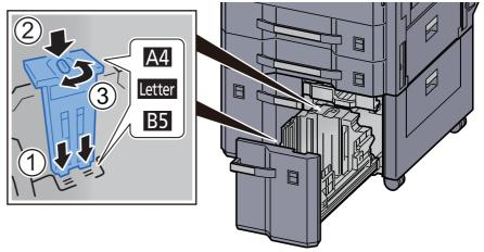
Make sure that the top of the Paper Size Guide (A) matches the paper size to be used, attach the clamp, and rotate the clamp to lock it.
