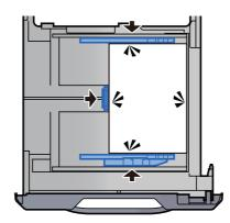
Insert the indication on the sheet so as to match the size and type of paper to be placed.
