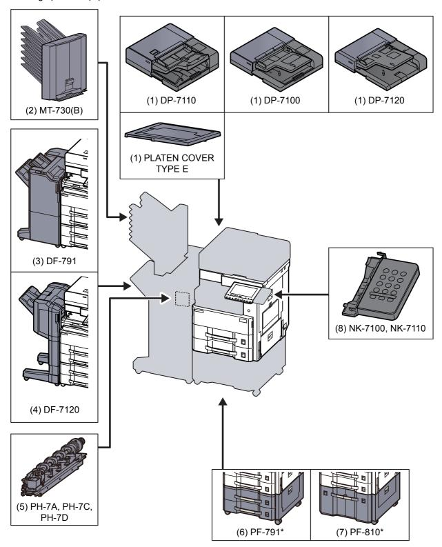
\* If the following option is installed, toppling prevention kit must be installed: PF-791, PF-810
