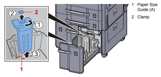
Insert the Paper Size Guide (A) into the slot (bottom of cassette) for the paper size to be used.
