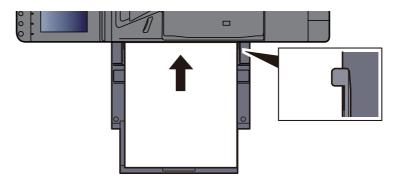
Insert the paper along the paper width guides into the tray until it stops.
