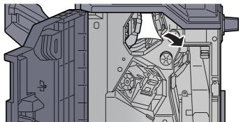
Q Return the conveyor guide (D4) to the original position.
