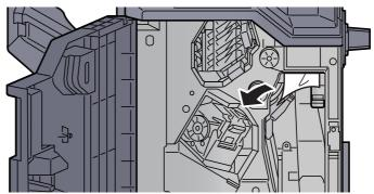
Q Return the conveyor guide (D1) to the original position.
