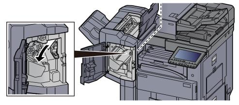
Q Return the conveyor guide (D1) to the original position.
