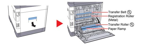
Wipe away the paper dust on the registration roller and the paper ramp using the cloth.
